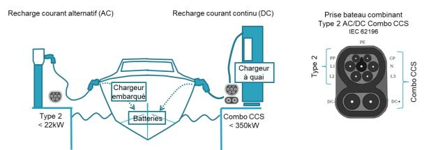
On the other hand, this standard allows direct current charging (DC+ and DC-), by installing the chargers at the quayside: saving space, weight saving and cost savings for the electric boat.
